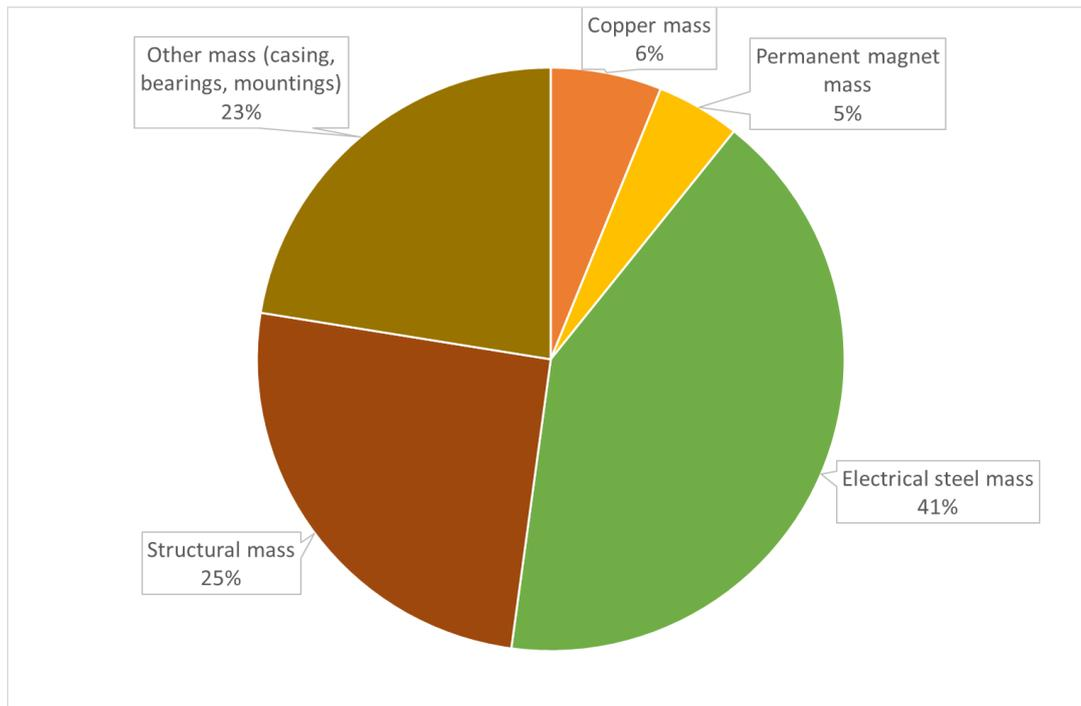
**Figure 3. Breakdown of mass for the direct drive generator.**
