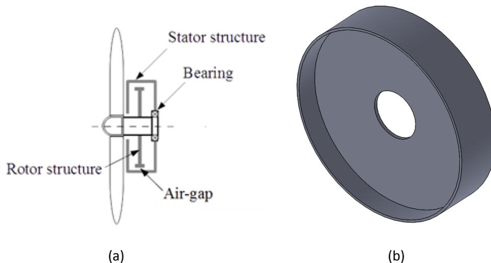
**Figure 2. (a) Generator structure [5]; (b) Rotor structure made of steel.**
