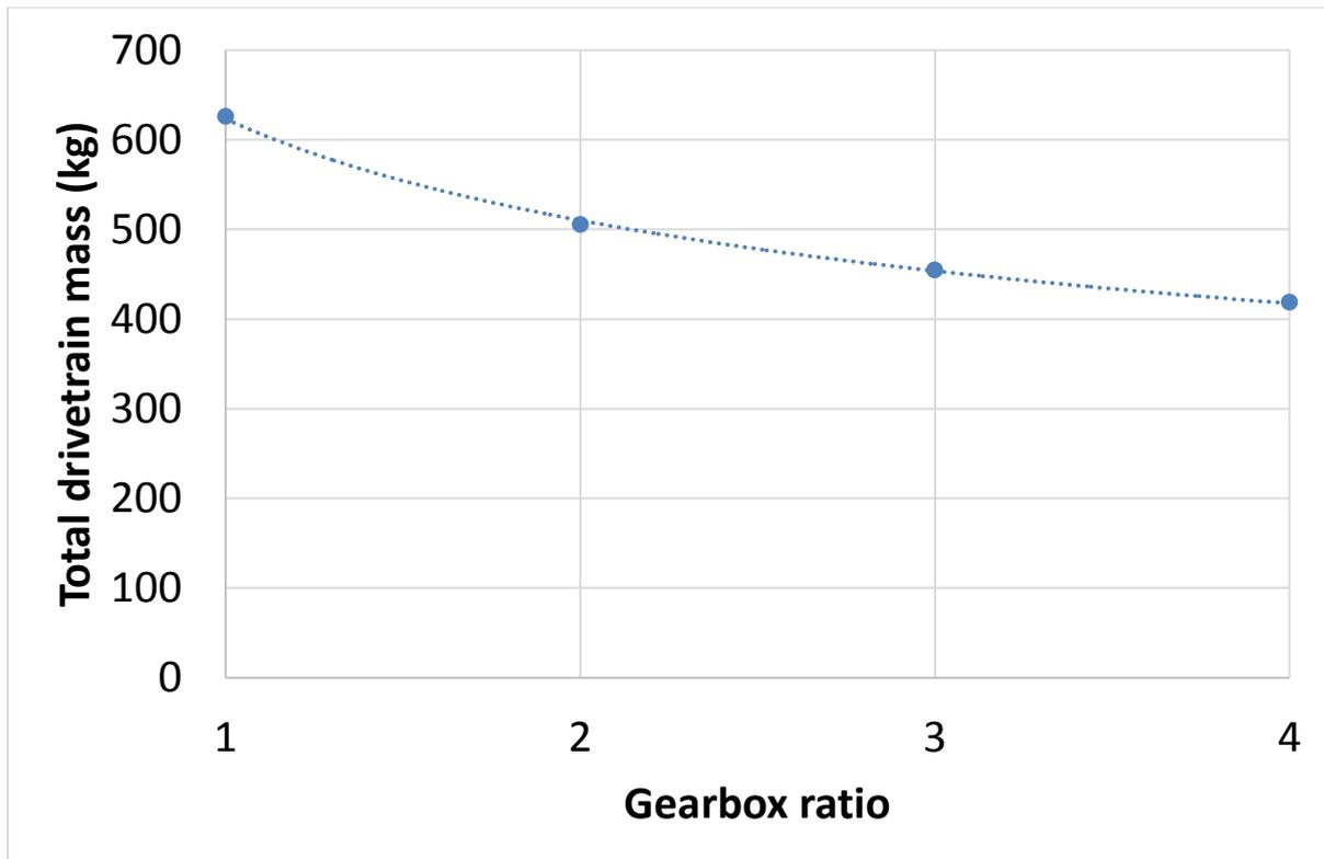
**Figure 4. Total drivetrain mass (mass of gearbox and generator) plotted against gearbox ratio.**
