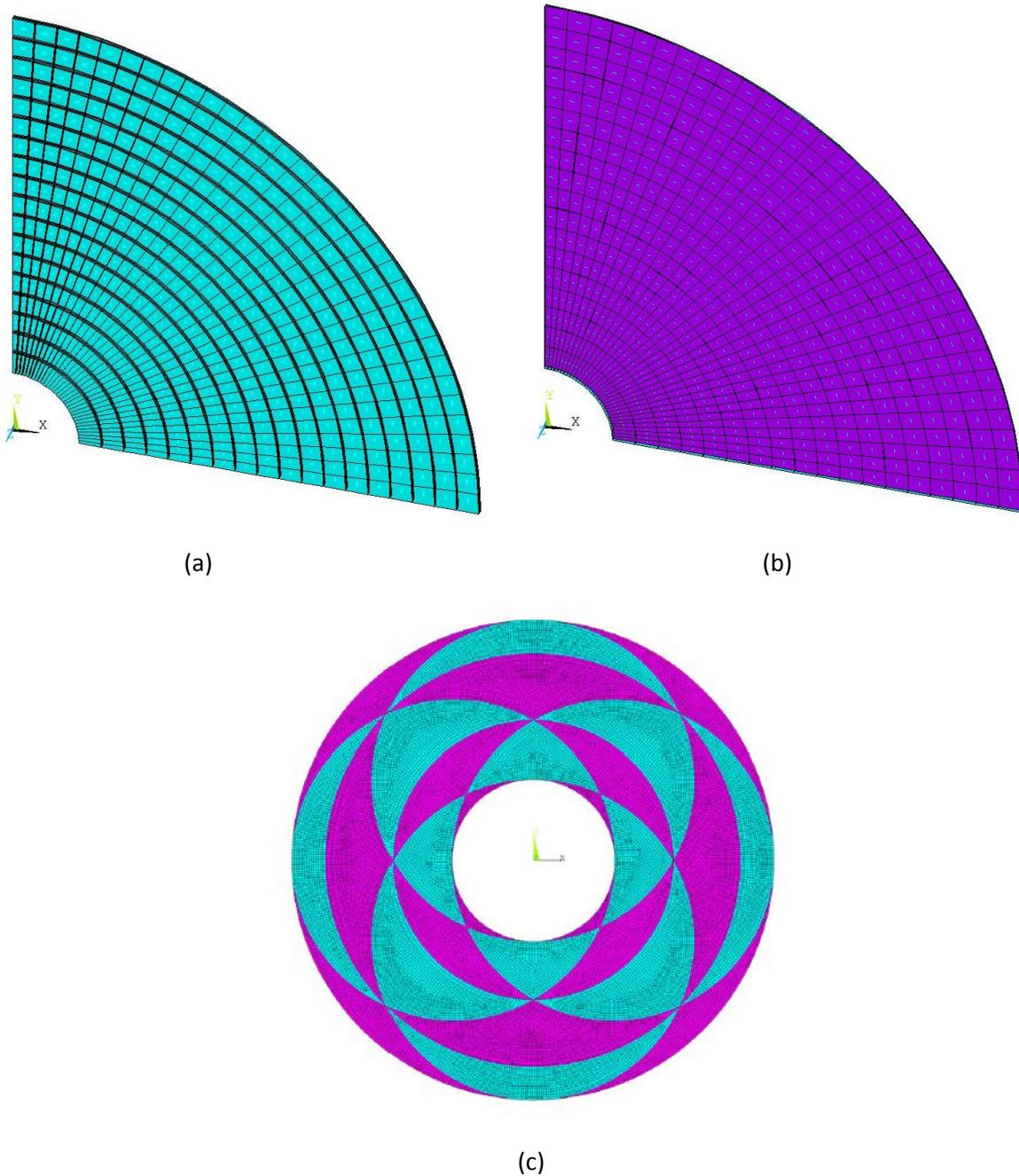
**Figure 5. (a) Conventional approach showing circumferential fibre orientation; (b) Conventional approach showing fibre orientation of reinforcing elements; (c) 4-unit disc (mosaic pattern fibre orientation) [4].**
