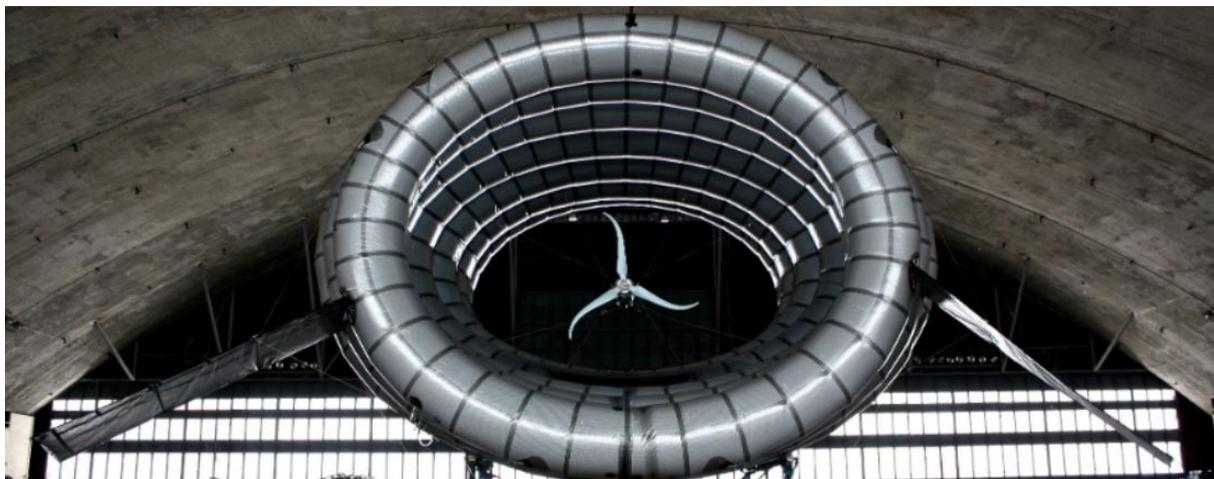
**Figure 1. Buoyant airborne wind turbine (BAT) [1]**
