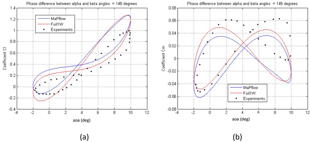
FIGURE 6: Comparison of predicted  $C_L$ ,  $C_M$  coefficients with measurements. Phase shift is  $135^\circ$
