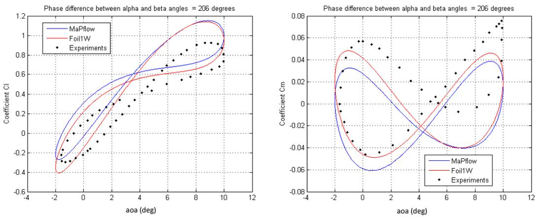
FIGURE 7: Comparison of predicted  $C_L$ ,  $C_M$  coefficients with measurements. Phase shift is  $206^\circ$
