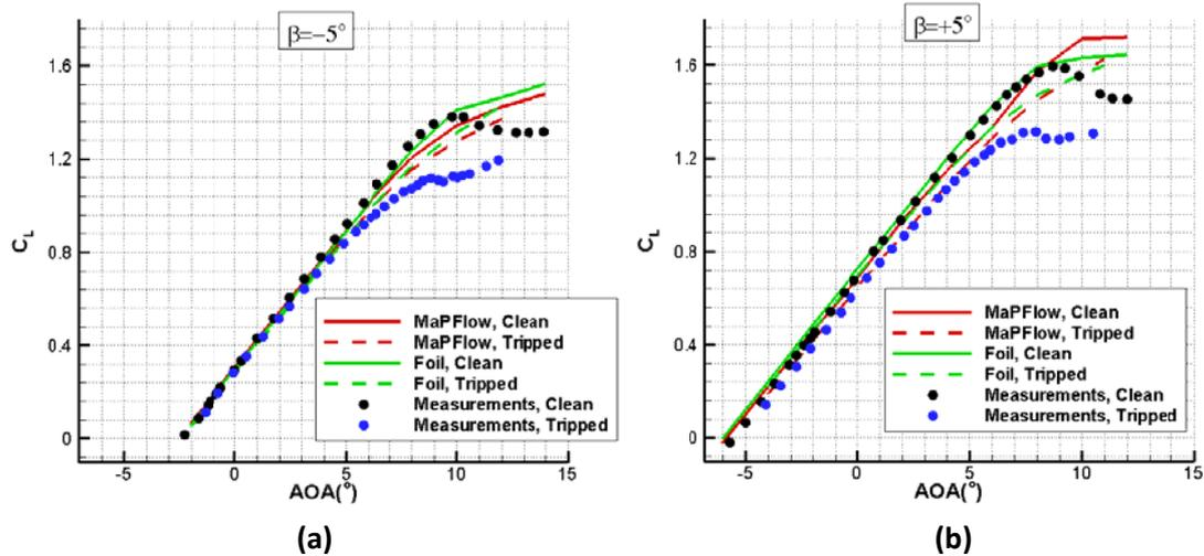
FIGURE 2:  $C_L$  polars for TE static flap, TL190-82 airfoil,  $Re=2.5 \cdot 10^6$ . (a) Flap= $-5^\circ$ , (b) Flap= $+5^\circ$ . Clean conditions correspond to free transition and tripped conditions correspond to fixed transition
