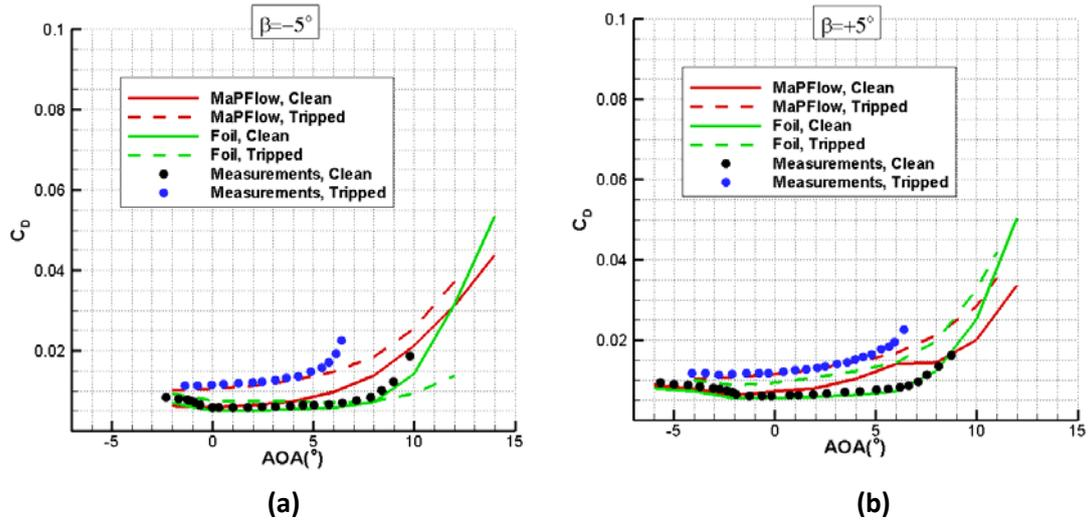
FIGURE 3:  $C_D$  polars for TE static flap, TL190-82 airfoil,  $Re=2.5 \cdot 10^6$ . (a) Flap=-5o, (b) Flap=+5o. Clean conditions correspond to free transition and tripped conditions correspond to fixed transition
