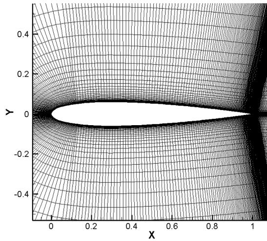
FIGURE 4: Computational mesh around the NACA0012 airfoil
