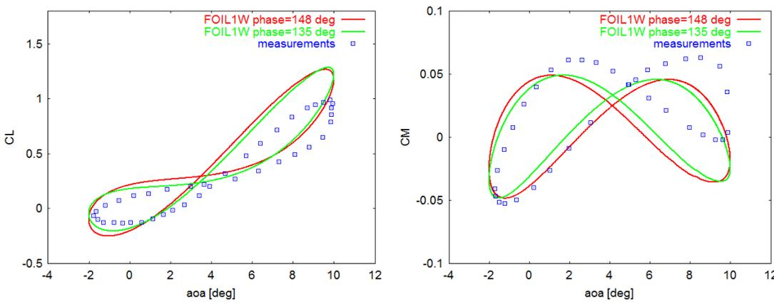
FIGURE 8: Modification in  $C_L$ ,  $C_M$  coefficients predicted by Foil when the phase shift is corrected from  $148^\circ$  to  $135^\circ$
