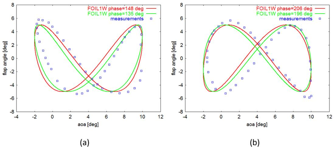
FIGURE 5: Theoretical and measured variation of the flap angle with the angle of attack for (a)  $\phi=148^\circ$  and (b)  $\phi=206^\circ$ . Nestor [6] suggested phase corrections from  $148^\circ$  to  $135^\circ$  and from  $206^\circ$  to  $196^\circ$  in order to fit the measured airfoil / flap relative motion
