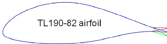
FIGURE 1: Articulated TE flap for the TL190-82 airfoil
