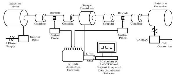
Figure 3: Test rig schematic diagram.
