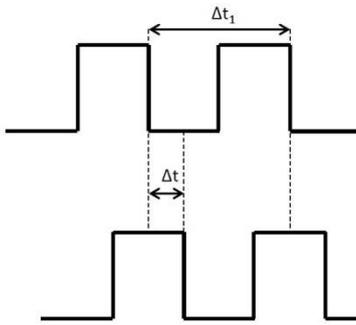
Figure 1: Typical pulse train, where  $\Delta t_1$  is the period and  $\Delta t$  is the phase shift.
