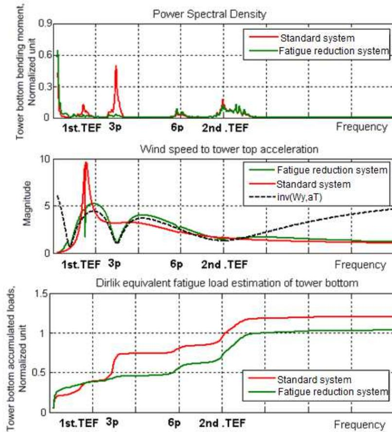
Figure 2: Top: PSD estimation of the tower bottom bending moment  $M_{TY}$ ; Middle: Magnitude bode plot of closed loop transfer function from wind speed  $\Delta v_{Wind}$  to tower top acceleration  $a_T$ ; Bottom: Accumulated fatigue estimation of  $M_{TY}$ .
