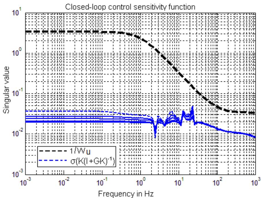
Figure 3: Singular values plots of the LPV closed-loop control sensitivity function for unstructured robustness analysis over the full-load operating range (blue), inverse weighting function (black).
