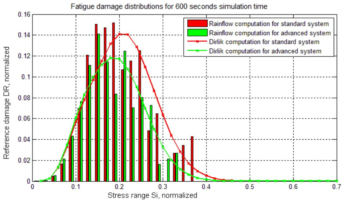
Figure 1: Distribution of fatigue damage contribution over stress range.
