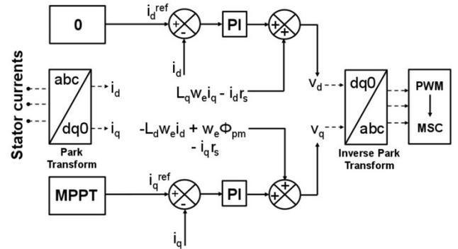
Figure 1: Schematic of machine-side controller.
