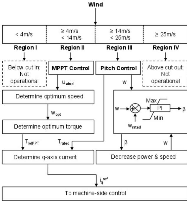
**Figure 2: Turbine control algorithm.**
