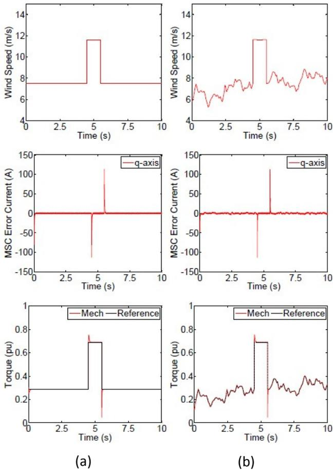
**Figure 3: Machine-side converter control response and torque for (a) steady profile (b) turbulent profile.**
