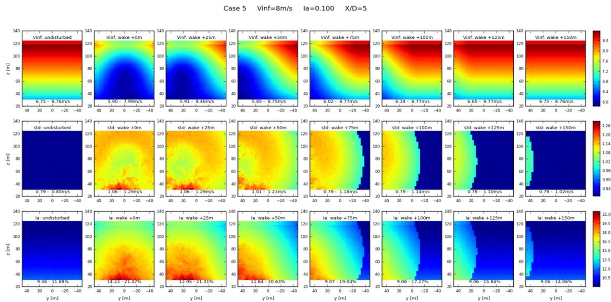
Figure 2 The wind average wind speed and turbulence field in a turbine area with different wake center locations. Free wind speed at hub height is 8m/s, ambient turbulence intensity is 10%, and  $x/D=5$ .
