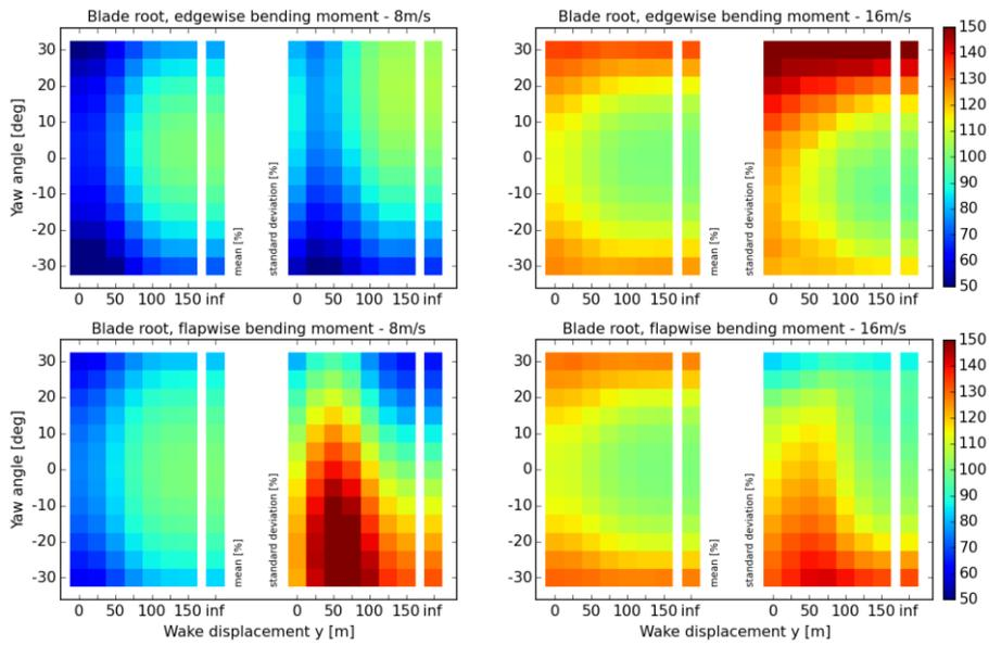
Figure 6 Edge- and flapwise bending moment at the blade root
