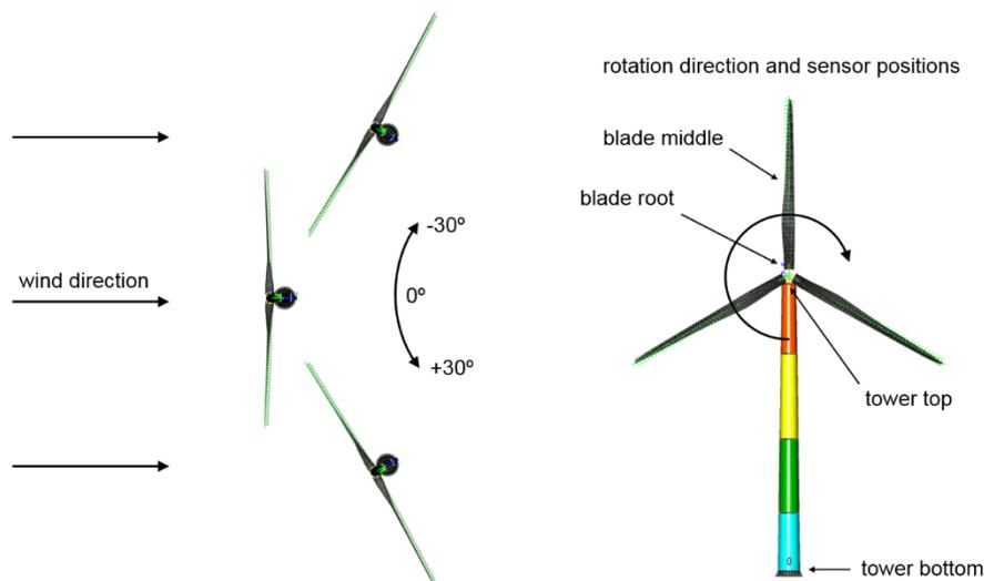
Figure 1 – Wind turbine model with direction references and sensor positions
