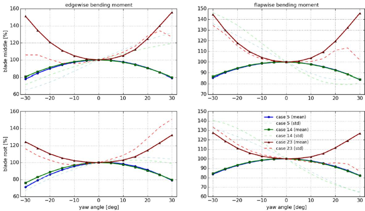
Figure 4 Edgewise and flapwise bending moments at 16m/s, 11 m/s, 8 m/s.
