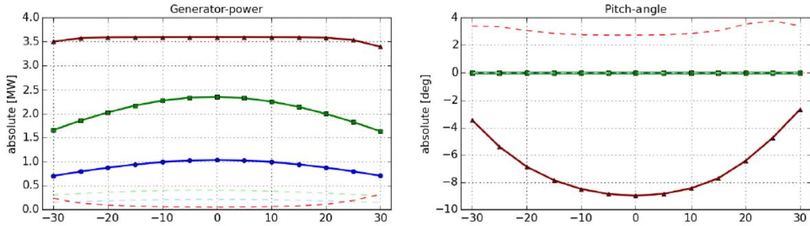
Figure 3 Generated power vs yaw angle for windspeeds 16m/s, 11 m/s, 8 m/s.
