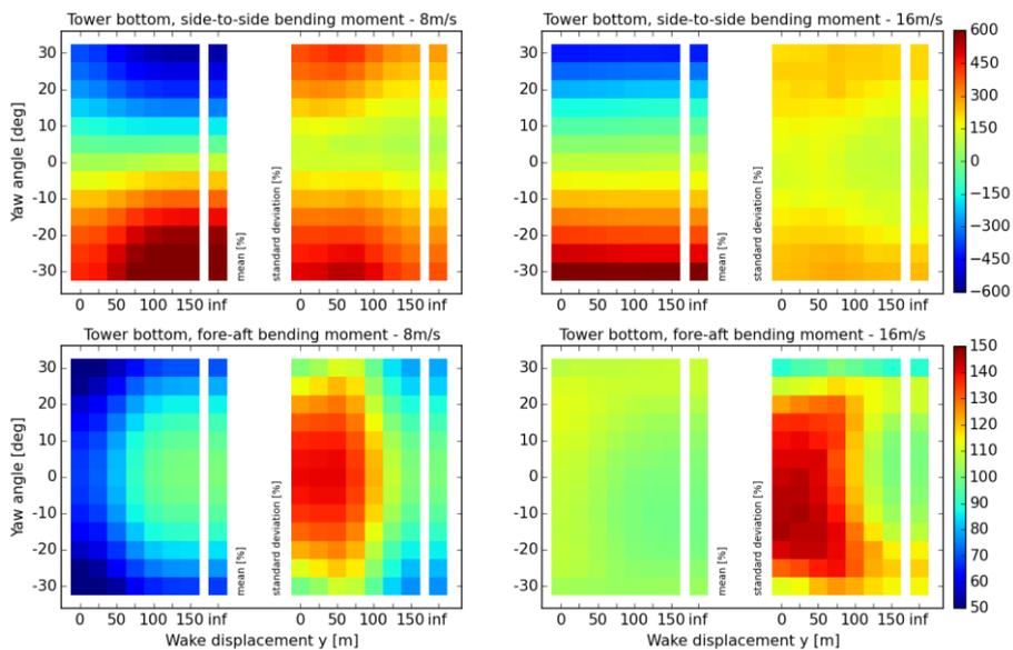
Figure 7 Side-to side and fore-aft bending moment at the tower bottom
