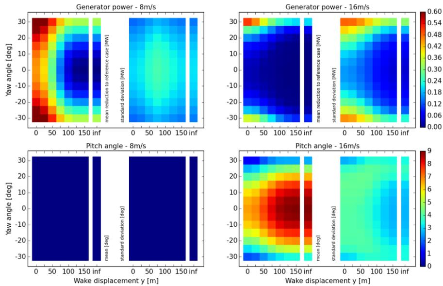
Figure 5 Generator power and pitch angle
