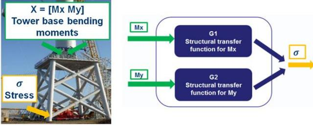
Figure2: MISO system workflow. A jacket critical point is studied taking into account bending moments at tower base. Structural transfer functions  $G_1$  and  $G_2$  are the dynamic characterization of jacket structural component.
