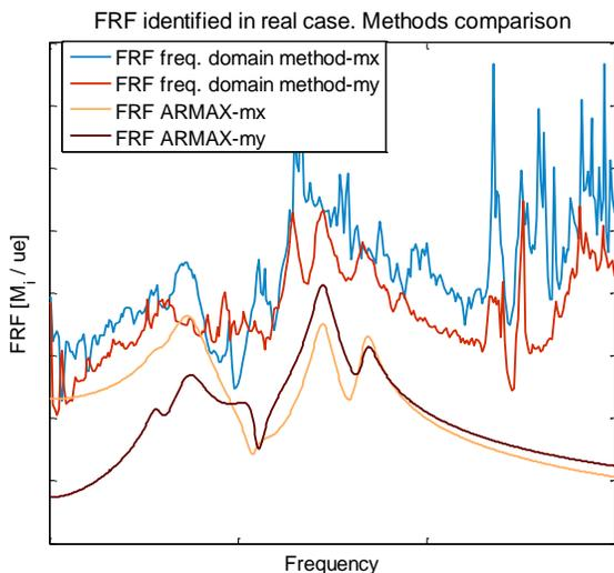
Figure5. FRFs in real case obtained by frequency domain method and time domain ARMAX model based. Results are smoother providing better modal
