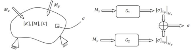
Figure1: In a general structural component loads are applied at different boundaries that produce a stress response in a critical point. Transfer function  $G_1$  and  $G_2$  characterize the local dynamics of structural component. Behavior. ARMAX representation is used to infer these transfer functions.
