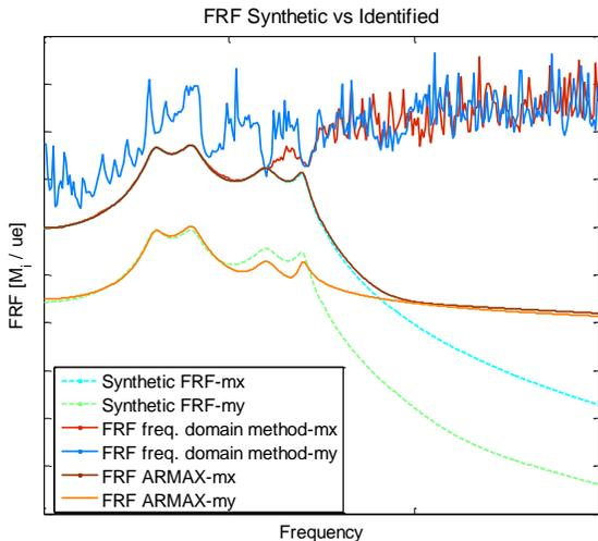
Figure4. FRFs synthetic obtained from known transfer functions. FRFs are obtained by classical method in frequency domain and time domain ARMAX model-based. (ue = micro strain, Mi = bending moment)
