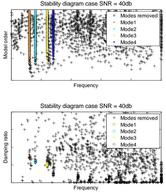
Figure3. Stability diagram in the case of synthetic data. Removed points by filtering step (black crosses). Modes drawn in colored circles.
