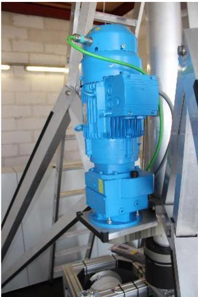
Figure 5: Mounting of the carousel motor
