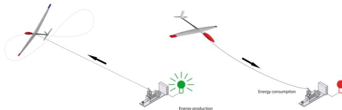
Figure 1: Example of a pumping cycle with a reel-in and reel-out phase as achieved by Ampyx Power [1].
