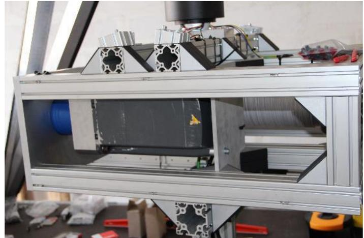
Figure 5: Mounting of the winch motor
