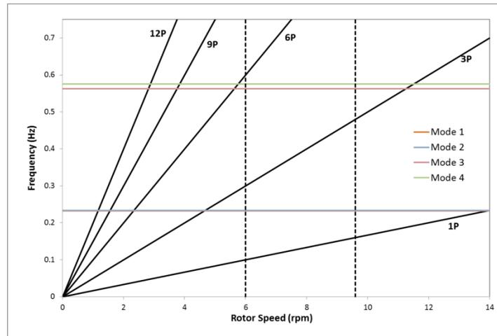
Figure 01. Campbell diagram of the proposed structure.
