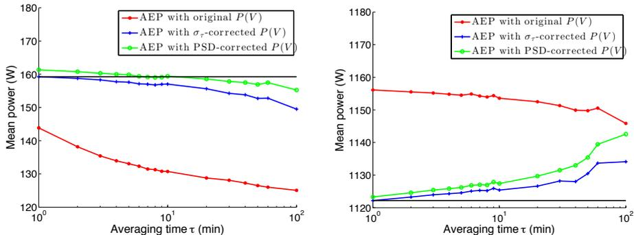
Figure 2: Mean power estimate as a function of the averaging time used. The line with circles shows the estimate with the power curve corrected from the power spectral density function. Site A is left, site B right.
