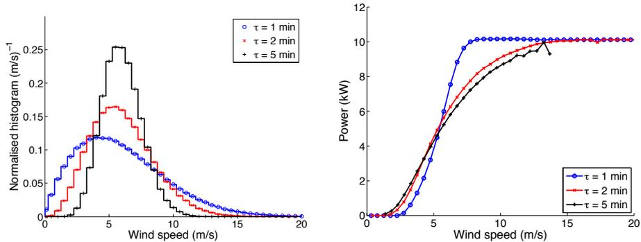
Figure 1: Effect of increased averaging times on the wind speed normalised histograms (left) and the power curve (right). The averaging times shown are 1 minute (circles), 2 minutes (crosses) and 5 minutes (pluses). The mean power output (integral of the product of the like curves left and right) is always the same.
