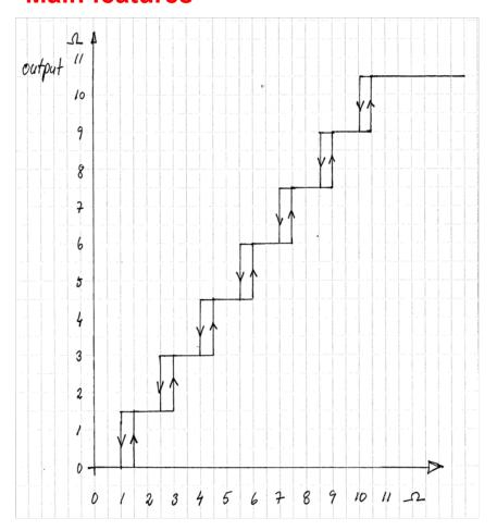
Step-Wise Switched Series Reactor FACTS: "Overload Power Flow controller".
