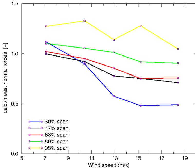
NREL Phase IV calc./meas. rotor(blade) loads, original model
