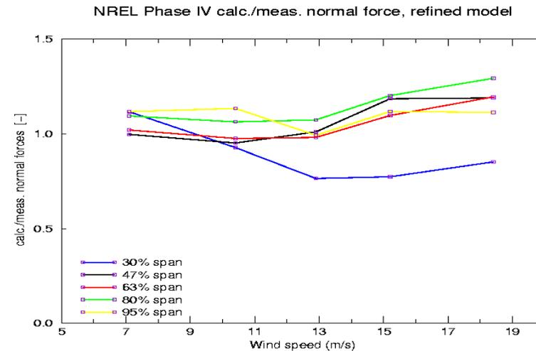
PHATAS modified modelling (derived from analysis of measurements <sup>1)</sup>)
